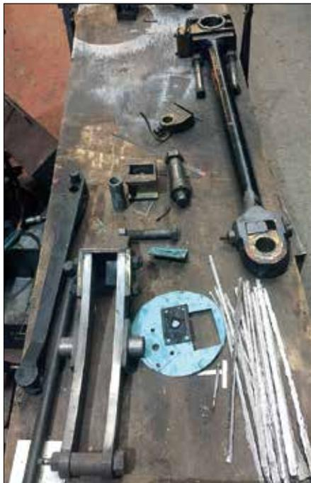
*Motion parts for the breakdown crane undergoing refurbishment.*
