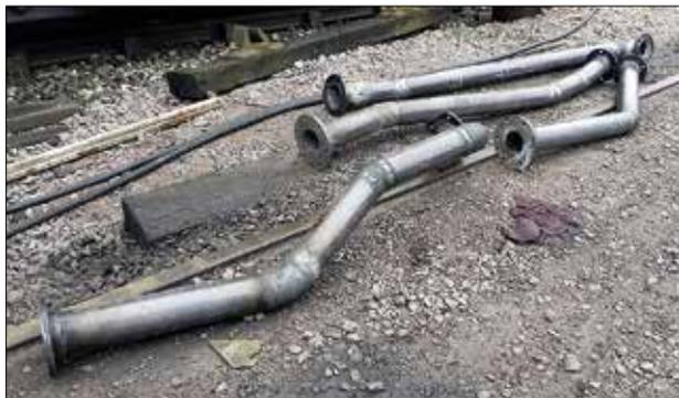
*The original steam supply pipe to the exhaust steam injector was removed from 45596 in the early 1960s. This is the new pipe assembly, and below, a view of it in situ bolted up to the inside cylinder casting.*
