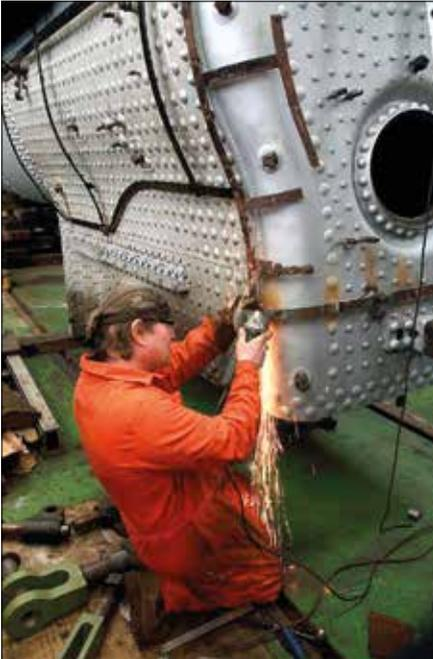
*45596's boiler at Tyseley on 7 March 2018 with the crinolines, on which the cladding is secured, in the course of fitting. photo: John Hillier*
