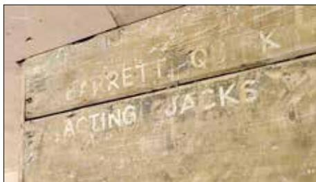
*Sign-written notice for Barrett quick-acting jacks. This indicated their location against one of the sliding door encasements in the tool space, when the vehicle was in used in breakdown trains.*
