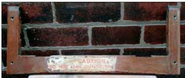
*One of the vent flap surrounds fitted above the corridor door droplights. Removal of layers of paint have revealed the BR era 'Caution...' labels.*
