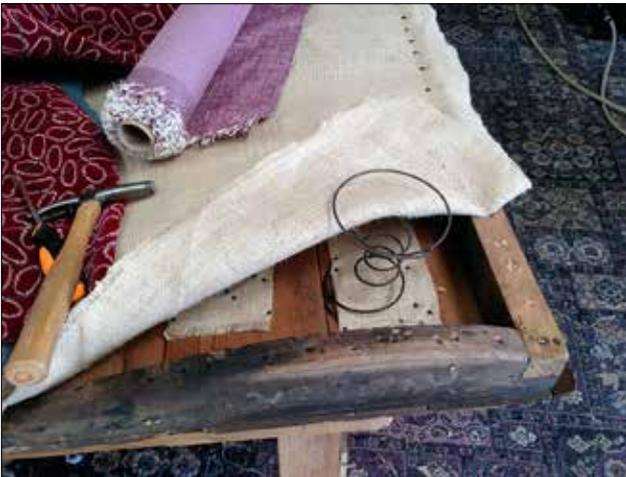
*One of the compartment seat backrests showing the arrangement of spring and webbing support, and the backing material, prior to covering with moquette.*
