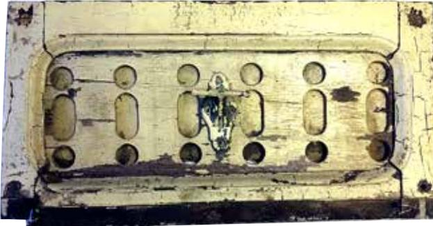
*This vent flap assembly, removed from one of the toilet cubicles in 2015, was fitted to LNWR coach No 117 when built in 1906.*
