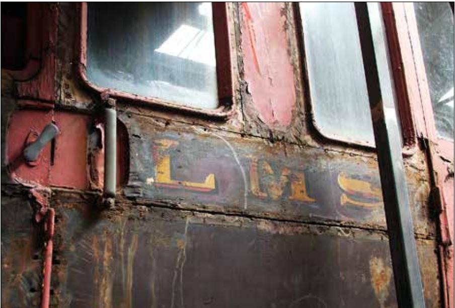
*The original waist panel as revealed on removal of the steel cladding.*
