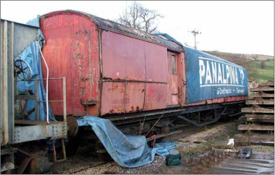
*Above - the Riding & Tool Van at Oakworth in 2012, showing some of the deterioration as a consequence of its 12 years stored beneath wagon sheets. Below at RRNE, Shildon, in September 2013 with the external refurbishment underway.*
